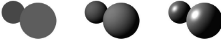
Figure 3.9: Spheres shaded using the Phong illumination model: a ambient reflection, b diffuse reflection, and c specular reflection. (By C. Garbe, University of Heidelberg.)
